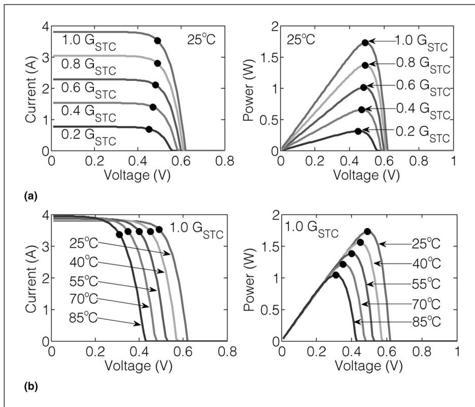
**Figure 1. PV cell output characteristics. (a) PV cell output under different solar irradiance. (b) PV cell output under different temperature.**
