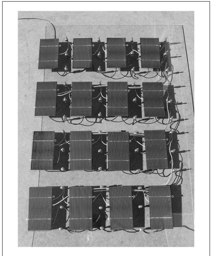
**Figure 6. Prototype of the fault-tolerant PV system.**
