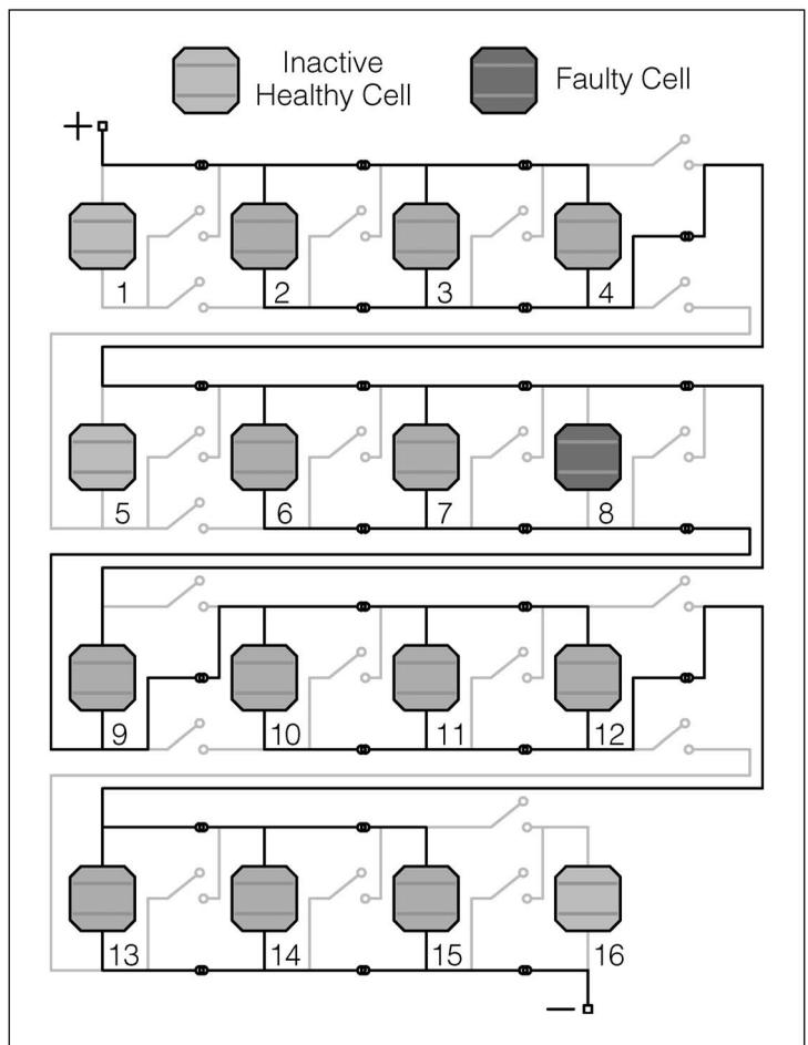
**Figure 4. Example of PV panel reconfiguration during fault detection and fault bypassing.**
