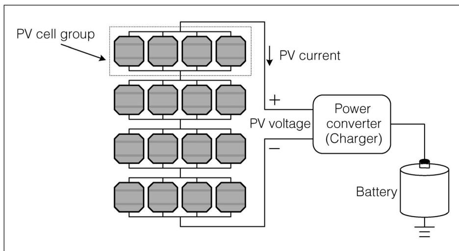
**Figure 2. Typical PV system architecture.**
