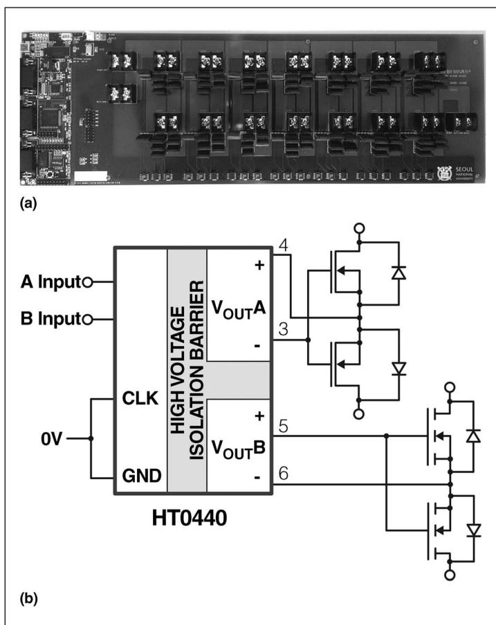
**Figure 7. (a) Computer-controlled programmable switch board, and (b) semiconductor realization of the switches.**
