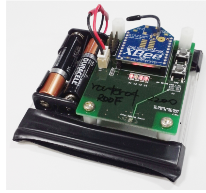
Figure 4: Zigbee-based solar sensor node to measure the solar irradiance.
