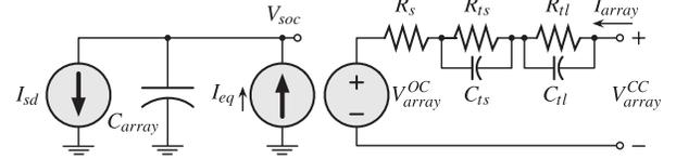
Fig. 3. Li-ion battery array equivalent circuit model.
