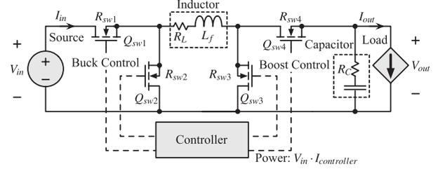
Fig. 2. Buck-boost switching converter circuit model.
