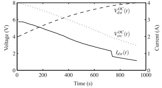
Fig. 6. Example of optimal time-unconstrained charge migration.
